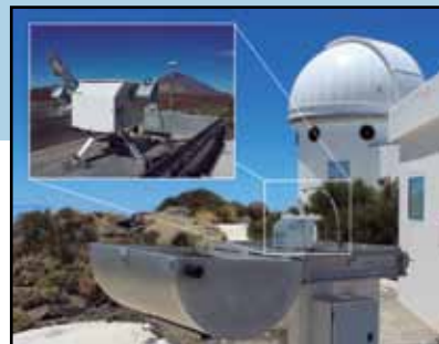
Fig 2.: Current setup of the automated solar tracker feeding solar light into the SONG spectrograph (back) by means of a fibre-optic system. A zoom of the azimuthal mount allows to clearly see the fibre assembling (right), the pyrhelometer and the active guiding (right). This project, so-called “Solar-SONG” is funded by the Severo Ochoa program at the IAC.
