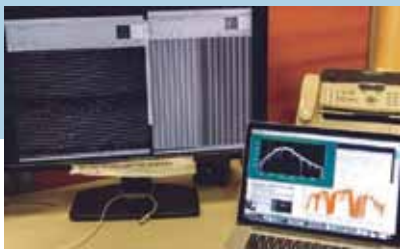
Fig. 1: The first light of GIARPS. The GIANO-B and HARPS-N spectra of HIP 029216 were achieved simultaneously and they appeared on the large monitor. The on-line pipeline provided the combined, reduced spectrum on the laptop screen.
