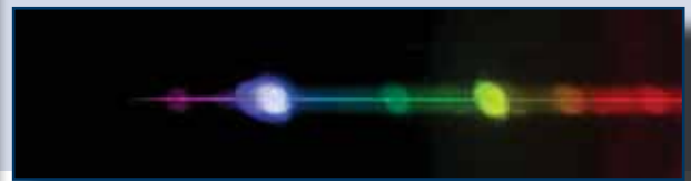
Fig. 3: A false-colour SPRAT "spectral image" of a planetary nebula (PN), taken shortly after commissioning of the instrument. The ionised nebula is seen in emission from a variety of atoms; the core of the dying star is seen as a horizontal strip of continuum emission.
