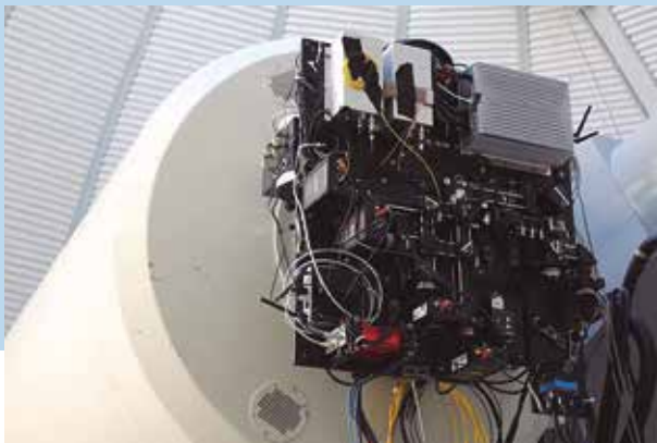
Figure 1: A quantum key receiver was installed at the OGS Cassegrain focal plane.
