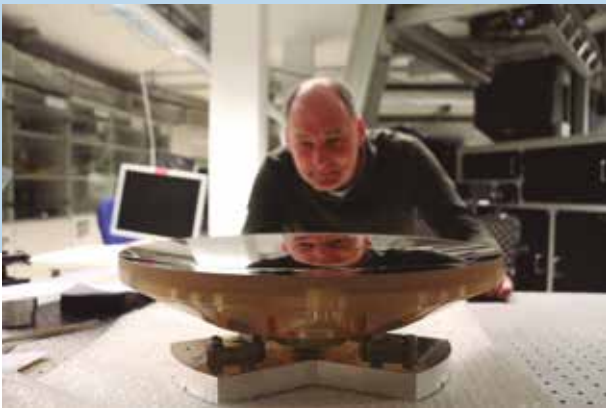
Figure 1: The new GREGOR secondary mirror (M2) during its incoming inspection in the optics lab.
