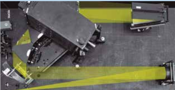
Figure 1: View of the light path of HORuS without the protective cover.
